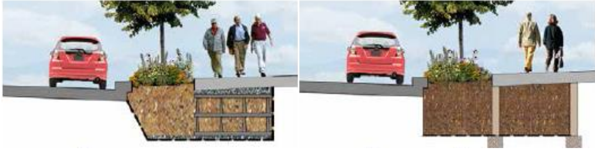
Figure 1-3. Stormwater tree well filter conceptual examples: modular suspended pavement system (left), column suspended pavement system (right). (Courtesy of Philadelphia Water Department)
